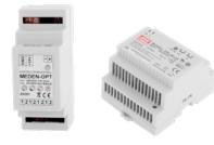
**The bus controller** is the power and communication module of the nurse call system. It provides power and organizes the communication flow on the system's bus. The controller is designed to work with the modules of the nurse call system. It has four bus connections with a load capacity of 150 mA each, and one communication connection for linking with other controllers in the system to increase the overall load capacity.
