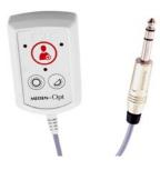
**The call pendant** is equipped with a 6.35 mm JACK plug and is used to initiate a call when connected to socket 39464. It features a "standby" light, which increases in intensity once a call is initiated. Additionally, it has two buttons for controlling lighting and is embossed with the Braille alphabet "SOS" above the call button. A mounting bracket is available for separate purchase.
